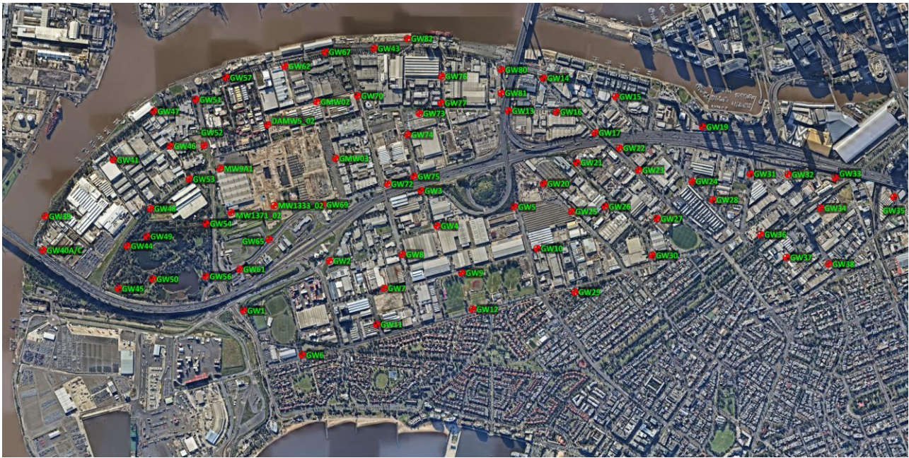
Figure 33 – Bores included in the new delineation of landfill impacts (Source nearmap 2020)
